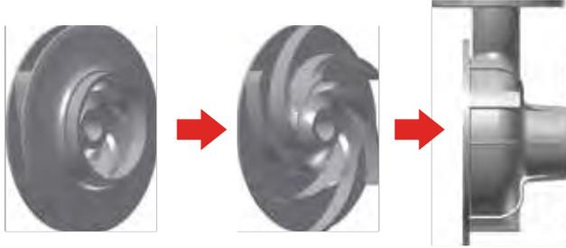
**ONLY ONE CASING EACH SIZE.** It can be used both for closed impeller (with wearing ring) and open impeller (with replaceable wearing plate): just with a few changes the pump can be adapted to new plant and process requirements. Pump casings are made by investment casting and they are electrochemically polished.
