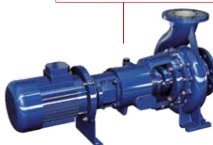
**EASY MAINTENANCE:** to build the whole pumps range (close-coupled, lantern bracket and on base plate execution) are necessary just 4 bearing housings and 6 lanterns. Oversized base-plates grant high stability; the lantern bracket execution avoids problems related to misalignment between pump and motor.
