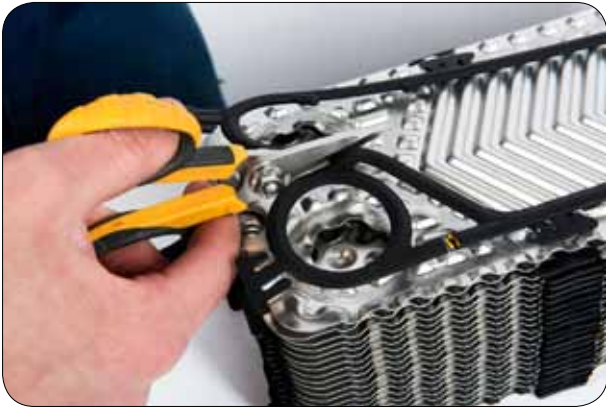
4.5 Cut two channel plate gaskets into half.
