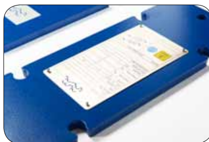
1.3 Drill four holes on the pressure plate to fit the holes in name plate and then put the name plate into position
