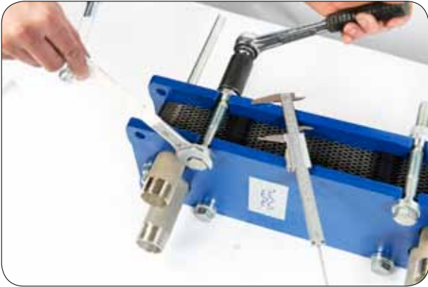
7.3 Tighten the plate heat exchanger to reach the A-measurement that is stated on the drawing of the heat exchanger.
