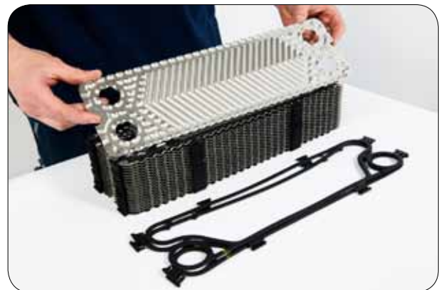
4.3 Repeat the above procedure to assemble the gasket onto the zero-holed end plate.
