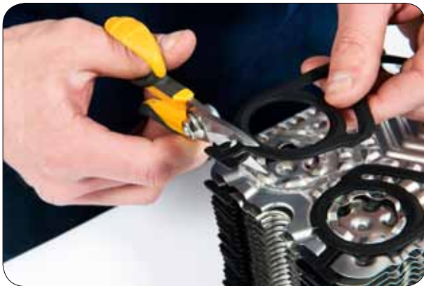
4.6 Cut off the clips from one of the half gaskets.
