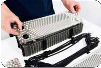
4.1 Assemble the gaskets onto the four-holed channel plates by using the fastening clips.
