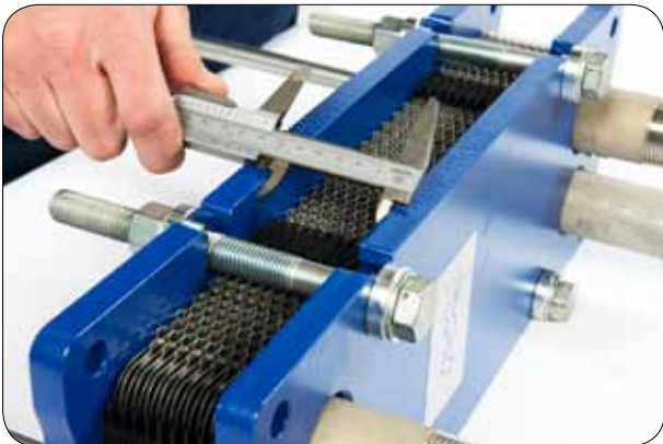
7.5. Check the A-measure and the parallel between the frame and pressure plate.
