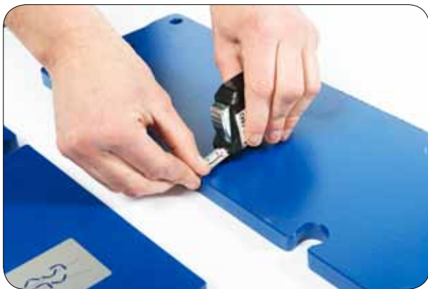
1.2 Mark the name plate position according to the location sketch
