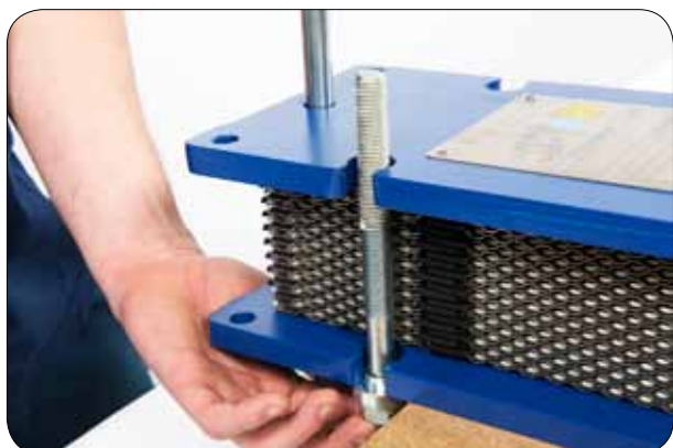
7.2 Assemble the tightening bolts, washers and nuts.
