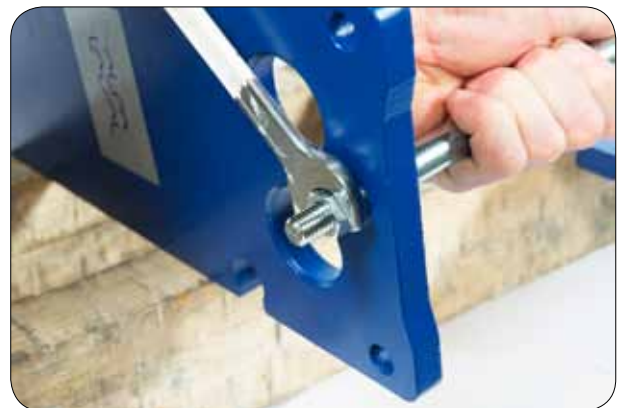
2.2 Assemble the carrying bar with help of nut and repeat the procedure to assemble the guiding bar.
