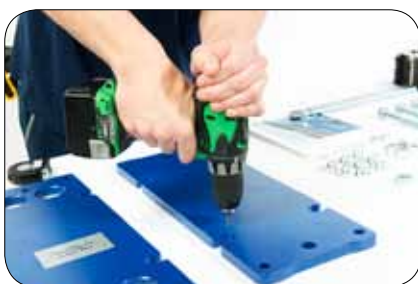
1.3 Drill four holes on the pressure plate to fit the holes in name plate and then put the name plate into position
