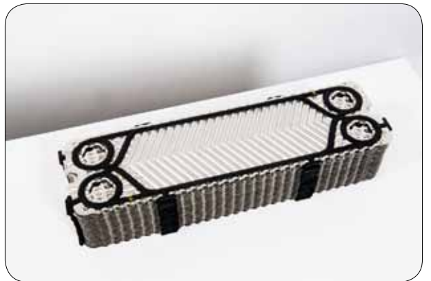
4.7 Combine the two half gaskets and assemble them onto the end plate.
