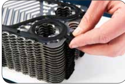
4.1 Assemble the gaskets onto the four-holed channel plates by using the fastening clips.
