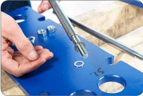
2.1 Place the carrying bar into the hole on the top of the frame plate.
