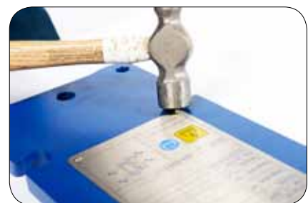
1.3 Drill four holes on the pressure plate to fit the holes in name plate and then put the name plate into position
