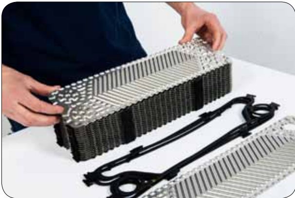
4.2 Repeat the above procedure to assemble the gasket onto the zero-holed end plate.
