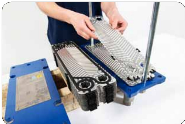
5.2 Assemble the plates according to the plate list of the heat exchanger.
