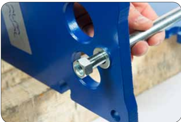
2.2 Assemble the carrying bar with help of nut and repeat the procedure to assemble the guiding bar.
