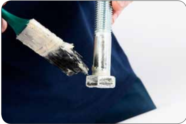
10.1 Grease the head of the tightening bolts and the washers.
