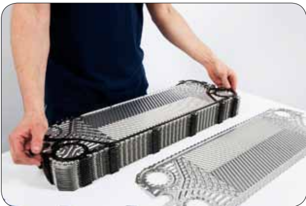
7.2 Repeat the above procedure to assemble the gasket onto the zero-holed end plate.
