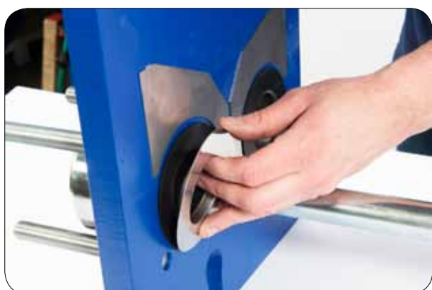
6.2 Assemble the pressed collars.
