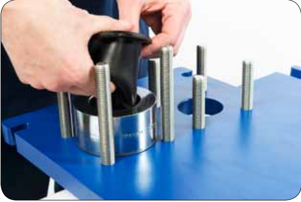
3.1. Assemble the rubber linings.
