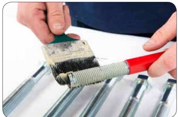
10.3 Grease the threads of the tightening bolts.
