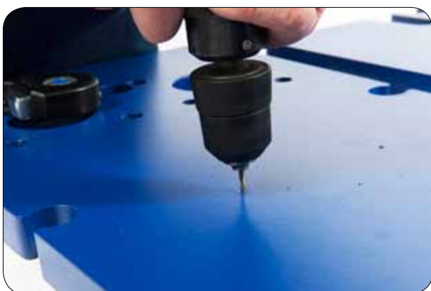
1.3 Drill four holes on the pressure plate to fit the holes in name plate.
