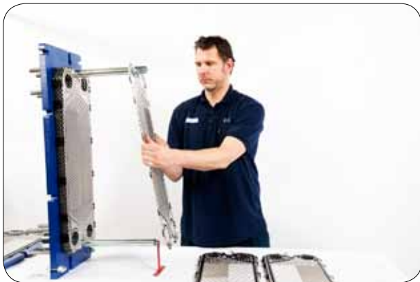
8.2 Hang the plates according to the plate list of the heat exchanger.
